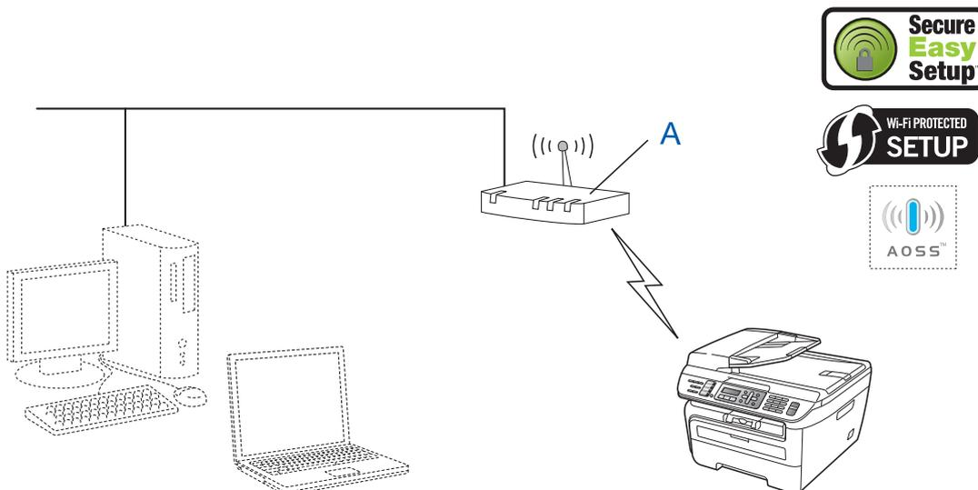
If your wireless access point (A) supports SecureEasySetup™, Wi-Fi Protected Setup™ or AOSS™, you do not need to use a computer to configure the machine. The access point (router) and your machine can automatically negotiate using the SecureEasySetup™ procedure. For instructions, go to page 25.
