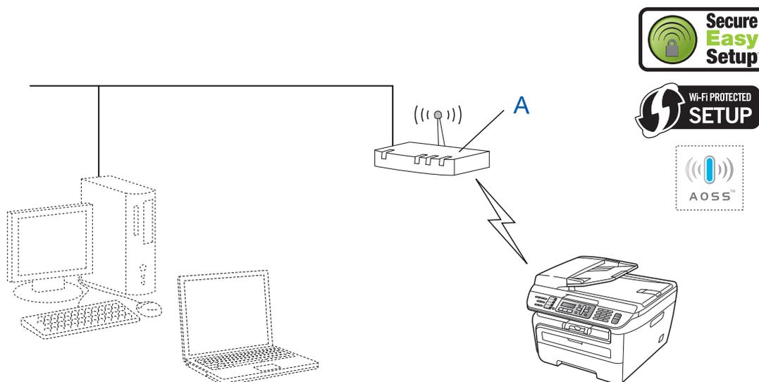
If your wireless access point (A) supports SecureEasySetup™, Wi-Fi Protected Setup™ or AOSS™, you do not need to use a computer to configure the machine. The access point (router) and your machine can automatically negotiate using the SecureEasySetup™ procedure. For instructions, go to page 39.
